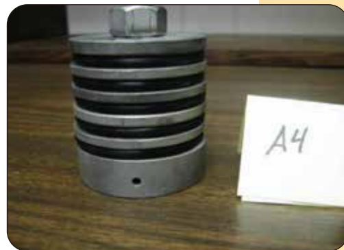
Figure 22 A4 Material installed on Tooling After Test
